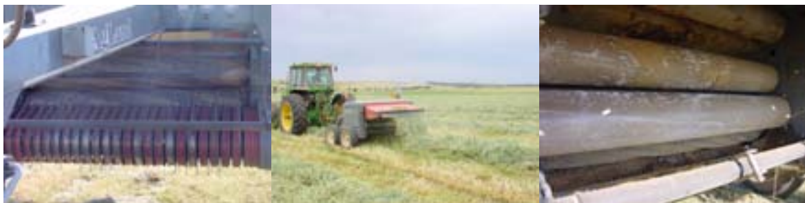
Figure 6 (L-R): Finger tynd pickup of Macerator 6610; Macerator 6610 in operation showing deposition of windrow; Rear fine tooth rollers
