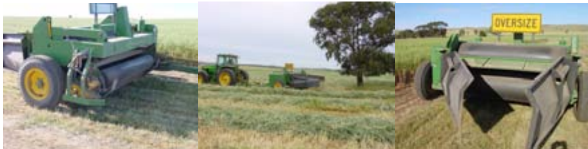
Figure 5 (L-R): Roller pickup system visible on Hydrasqueeze; Hydrasqueeze in operation showing deposition of windrow; rear view of Hydrasqueeze showing adjustable rear wings
