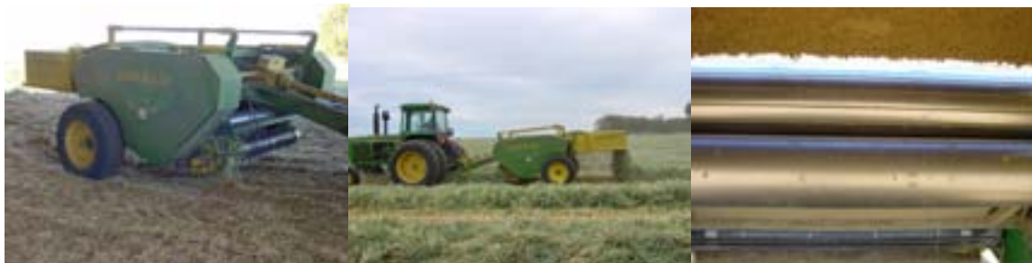
Figure 4 (L-R): Front view of Haymax showing finger tynd pickup; Haymax in operation showing deposition of windrow; roller system in Haymax
