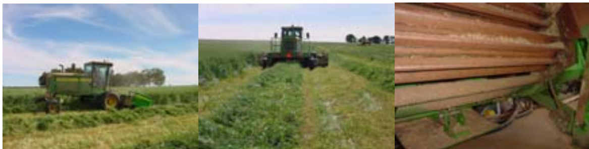
Figure 1(L-R): Side view of SP mower conditioner; rear view of mower conditioner; roller design of mower conditioner.
