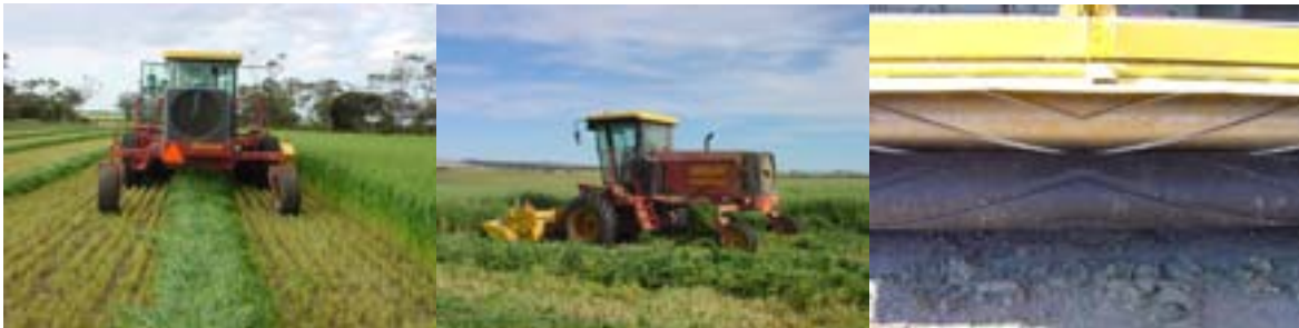
Figure 3 (L-R): Rear view of New Holland SW340; side view of New Holland SW340; interlocking roller system for New Holland SW340
