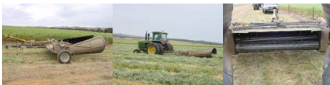
Figure 7 (L-R): Side view of Recon300; Recon 300 in operation; rear view of Recon300, showing rollers and adjustable rear flaps
